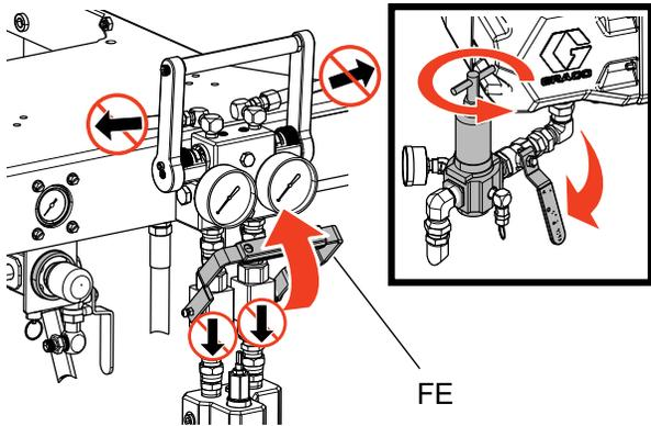
8. Close the solvent pump air valve (DA). Trigger the gun to relieve pressure. Close the solvent flush valve (FD) after relieving the pressure.
