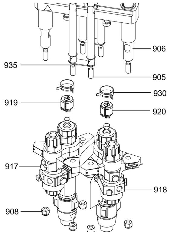
6. Use a wrench to hold the tie rod (905, 906) flats to keep the rods from turning. Unscrew the nuts (908) from the tie rods and carefully remove the displacement pump (917 or 918) and lower straps (935).
