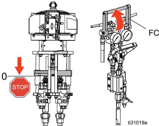
3. Close the motor air valve (MA) and turn the air regulator (MB) counterclockwise. Lower to open the circulation handle (FC).
