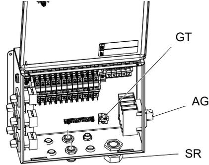
8. Verify that all items are connected properly as shown below, then close the electrical enclosure door.
