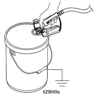
6. Engage the trigger lock. Install the tip on the gun.
