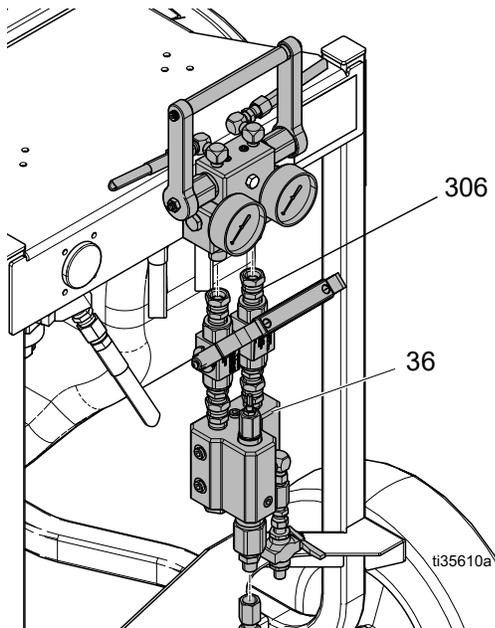
2. Connect "A" and "B" material hoses to the fluid circulation manifold (35) using necessary adapter fittings (supplied with heated hose).
