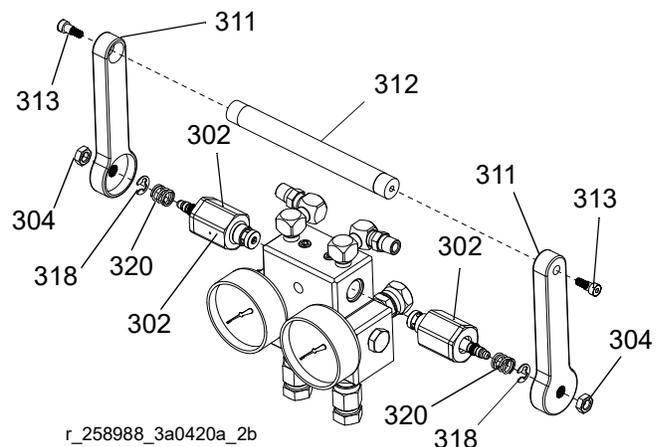
4. Unscrew both over pressure relief valves (302) from the manifold.
