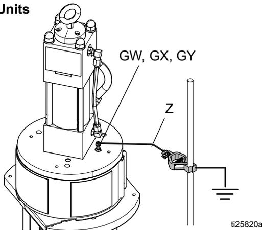
Loosen grounding lug locknut (GW) and washer (GX). Insert ground wire end (Z) into lug (GY) slot and tighten locknut securely. Connect ground clamp to a true earth ground.
