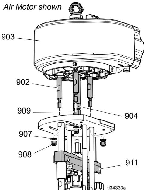
6. Place a wrench on adapter rod (904). Use tool (69) to loosen the serrated yoke nut (909) that holds the air motor (903) above the yoke (911).
