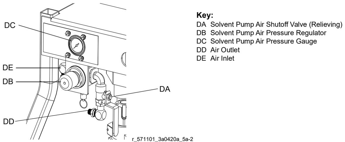
**FIG. 6: Solvent Flush Pump Kit Air Controls**
