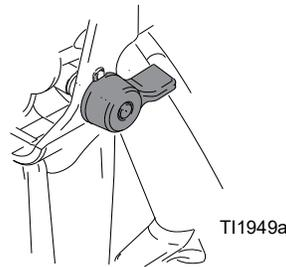
3. **XP Systems:** Turn the main pump air regulator (MB) fully counter-clockwise to shut off.
