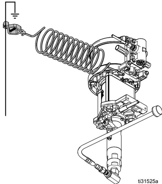
**Air and fluid hoses:** use only static dissipation type hoses with a maximum of 300 ft (91 m) combined hose length to ensure grounding continuity. Check electrical resistance of hoses regularly. If total resistance to ground exceeds 29 megohms, replace hose immediately.
