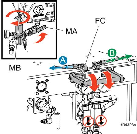
2. Lift to close the circulation handle (FC) when the pump is at the bottom of the stroke.
