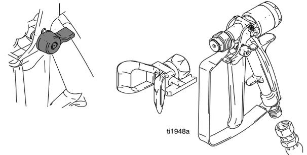
6. Open the solvent flush valve (FD)
