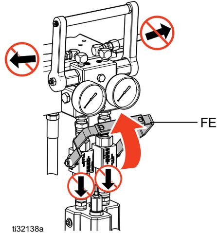
9. Remove pump fluid filters, if installed, and soak in solvent. Clean and replace the filter cap. Always replace the filter o-rings. See your Xtreme pump manual.
