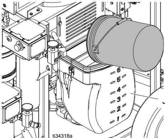
3. Fill the A and B hoppers with proper materials. Fill the A side (blue) with major volume of material; fill the B side (green) with minor volume of material (unless 1:1 mix ratio).
