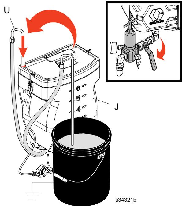
10. If using heaters, heat fluid throughout system before spraying. See **Recirculate Prior to Spraying or Re-Prime After a Pump Runs Dry**, page 34.
