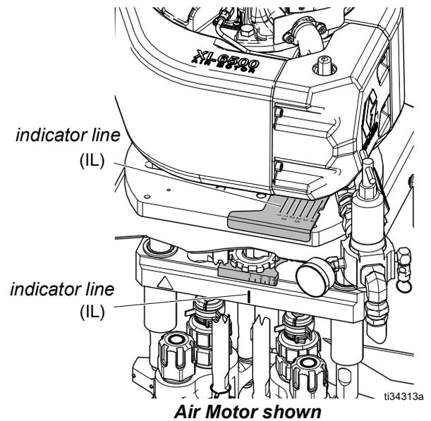
2. Verify that the motor position is adjusted correctly for that mix ratio (refer to the image above). If not, follow the **Change Motor Position** procedure on page 26.
