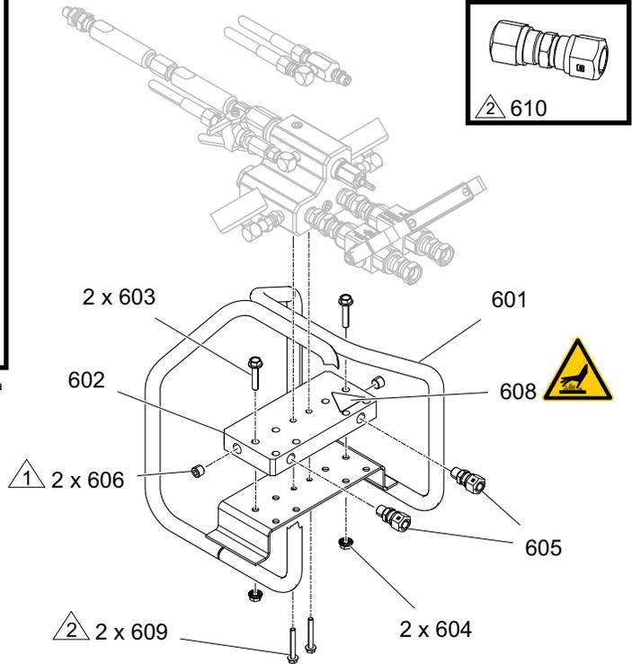
① Apply thread sealant to all non-swiveling pipe threads.
