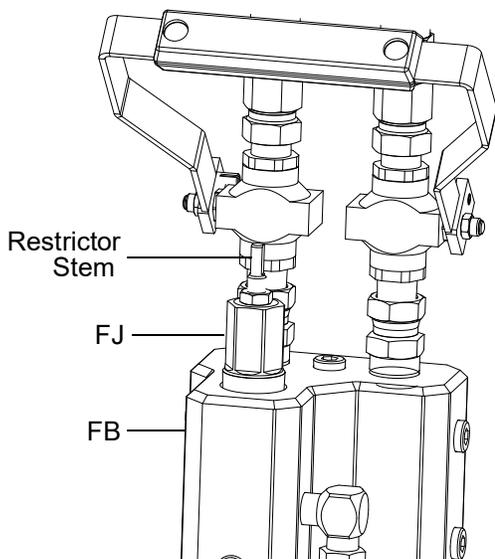
If the mix manifold (FB) is mounted on the machine, you do not need to adjust the restrictor. Leave the restrictor stem open two turns minimum from fully closed.
