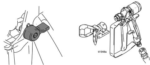
8. Disengage the trigger lock and trigger the gun into a grounded metal pail while holding against a pail. Use a pail lid with a hole to dispense through. Seal around the hole and gun with a rag to prevent splash back. Be careful to keep fingers away from the front of the gun.
