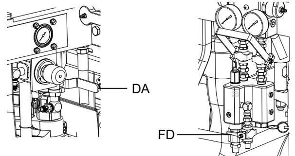
5. Open the solvent pump air valve (DA). Slowly turn the solvent pump air regulator (DB) clockwise to increase air pressure.
