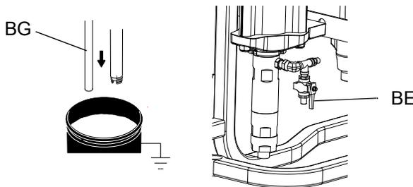
4. Open the solvent prime valve (BE) on the solvent pump (BA) outlet.
