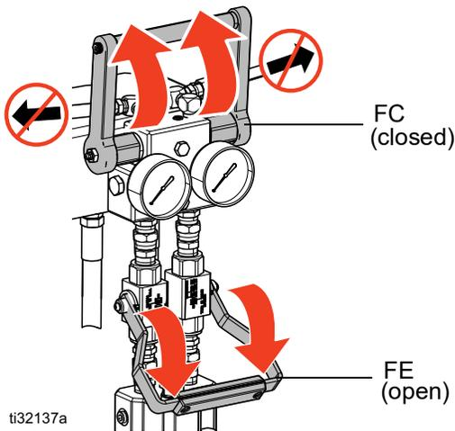
5. Open the motor air shutoff valve. Increase the air regulator pressure to 20 psi (1.9 bar).
