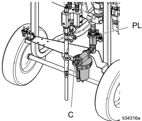
2. Remove plugs (PL) as necessary for solvent pump and feed supply pump air hoses. See pump manuals for setup instructions.
