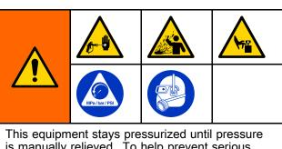
This equipment stays pressurized until pressure is manually relieved. To help prevent serious injury from pressurized fluid, such as skin injection, splashing fluid and moving parts, follow the Pressure Relief Procedure when you stop spraying and before cleaning, checking, or servicing the equipment.
