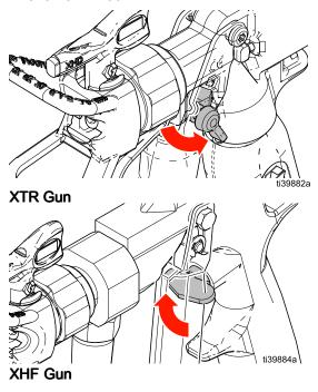
2. Pull pressure adjustment knob (H) out and turn counterclockwise until it stops. Push the knob in to lock.
