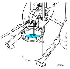
5. Use two wrenches to loosen the hose, then disconnect the hose from the outlet check valve housing.
