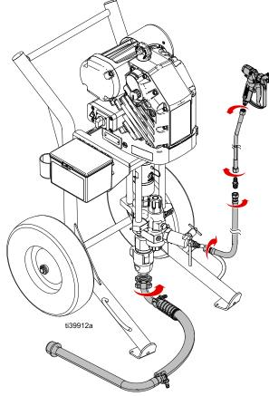
**NOTE:** Maximum suggested length is 6 ft (1.8 m), minimum suggested inner diameter is 1 in. (2.5 cm).
