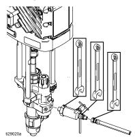
6. Use a wrench to loosen the outlet check valve, then remove the outlet check valve from the pump lower.
