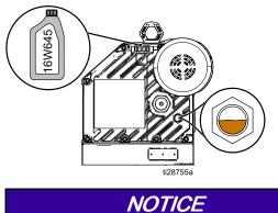
Only use oil with Graco part number 16W645. Any other oil may not lubricate properly and can cause damage to the drive train.
