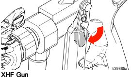
5. Hold gun firmly against a grounded metal pail. Trigger the gun.
