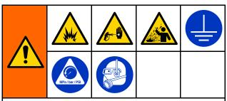
To avoid fire and explosion, always ground equipment and waste container. To avoid static sparking and injury from splashing, always flush at the lowest possible pressure.
