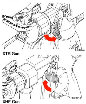
7. **Drain fluid:** Place the drain tube in a grounded waste pail. Slowly open fluid drain/purge valve (C), and drain fluid into a waste pail.
